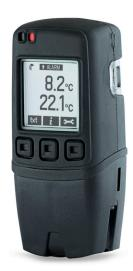
This standalone data logger measures and stores more than 250,000 temperature readings from two K, J or T-type thermocouple probes at a resolution of 0.1°C (0.2°F). It comes supplied with two K-type thermocouples capable of measuring from 0 to 200°C (32 to 392°F).
