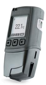
This standalone data logger measures and stores more than 250,000 temperature readings from a K, J or T-type thermocouple at a resolution of  $0.1^{\circ}$ C ( $0.2^{\circ}$ F). It comes supplied with a K-type thermocouple capable of measuring from 0 to 200°C (32 to 392°F).
