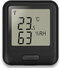
The EL-WiFi-TH measures the temperature and humidity of the environment in which it is situated. This sensor is typically accurate to  $\pm 0.3^{\circ}C/\pm 0.6^{\circ}F$  (+5 to  $\pm 60^{\circ}C/\pm 1$  to  $\pm 140^{\circ}F$ ) and  $\pm 2.0\%$ RH (20 to 80%RH @ 25°C). Data is streamed wirelessly over any WiFi network and can be viewed on a PC using free software or on the FilesThruTheAir<sup>TM</sup> Cloud.
