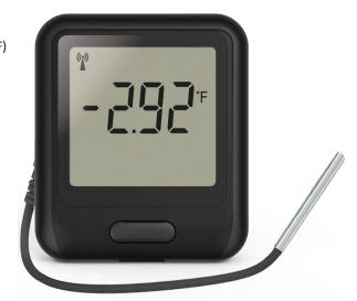
During configuration, the sensor will search for an existing wireless network whilst physically connected to the PC. It can then be placed anywhere within range of the network. If the sensor temporarily loses connectivity with the network, it will log readings until it is able to communicate again with the PC application or EasyLog Cloud (max 30 days at 10 second sample interval).
